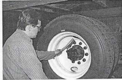
P6-2 Remove rust and road dirt from the wheel studs with a wire brush.
