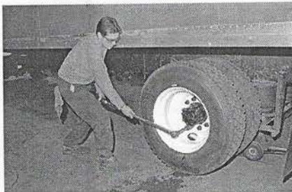
P6-7 Tighten the wheel nuts in sequence in three stages using a torque wrench. First-stage torque value should be 50 ft.-lb. Second-stage torque should be between 50 and 80 percent of the final torque value. Final torque values are listed at right.
