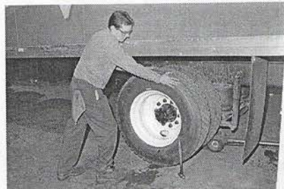
P6-8 As a final step, check the wheel runout by rotating the wheel through a full revolution. Do not attempt to correct a runout problem by loosening and retorquing the nuts: disassemble the wheel assembly and locate the problem.
