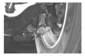
P9-5 Mount the dial indicator on the front axle I-beam with the dial indicator plunger touching the inner side of the lower end of the knuckle. Zero the dial indicator. While a helper moves the bottom of the tire inward and outward, observe the dial indicator reading. If the dial indicator reading exceeds the specified kingpin bushing movement, replace the lower kingpin bushing.
