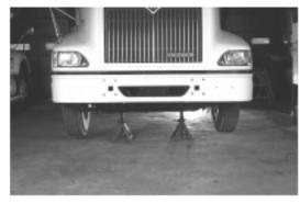
P9-2 Lower the vehicle so that it is supported securely on safety stands with the front tires still off the shop floor.
