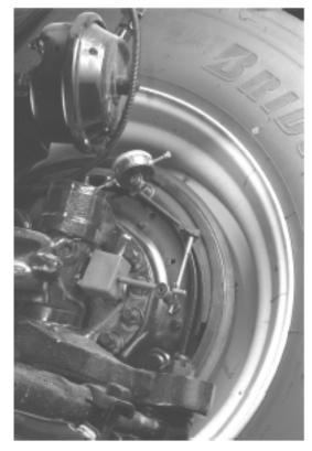
P9-6 Mount the dial indicator on the axle I-beam and position the dial indicator plunger on top of the upper knuckle joint cap.
