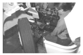
P9-7 Use a pry bar to force the steering knuckle downward. Check the reading on the dial indicator.
