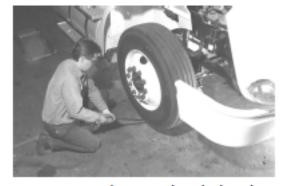
P9-8 Next, observe the dial indicator reading while a helper uses a large pry bar to lift upward on the tire and wheel. If the dial indicator reading exceeds the truck manufacturer's specifications, remove the steering knuckle and inspect the thrust bearing. Replace this bearing if necessary and install the required shim thickness.
