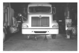
P9-1 Apply the parking brakes, block the rear wheels, and use a floor jack to raise the front axle until the tires are off the shop floor.
